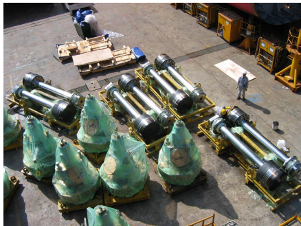
Main pistons and cylinder covers (still covered and exhaust cage closed by plate)
