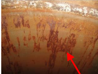
Heavily corroded: Cylinder liner and piston crown. At last the parts could be pulled or reached to be cleaned and judged for further procedure (replacement).
