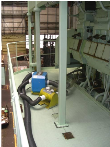
Sample picture of the installation of a Munters M120 dehumidifier
