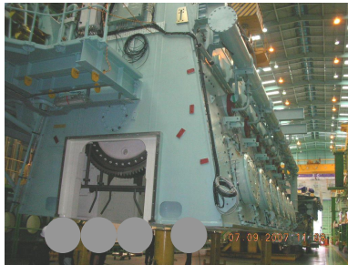
Column at cleaning stage. Cleaning solvent (white spirit) is used.
