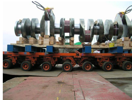
Crankshaft delivered as single part. Already cleaned of corrosion protector by solvent and ready for bedplate assembling. Crank-throw journals protected with rubber and steel plates (8mm thick).
