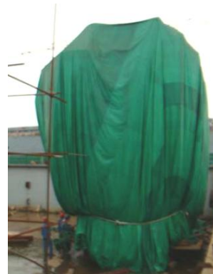
Engine stored outside and covered with a waterproof tarpaulin.
