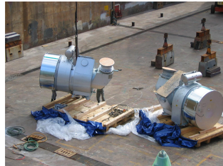
Turbocharger prepared ( openings closed by wooden plates)
