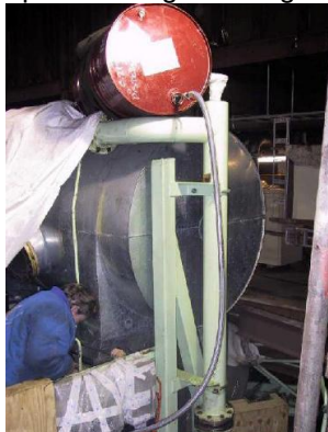
Additional lubrication oil tank connected to the fuel rail to keep it under constant static pressure.
