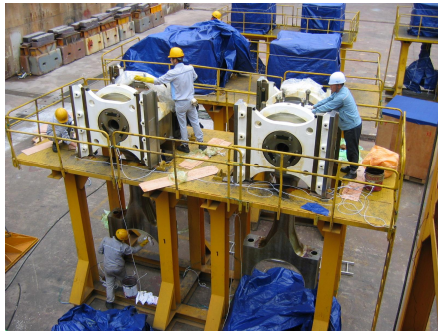
Connecting rods at cleaning stage at shipyard. The sea-trial date is fixed.
