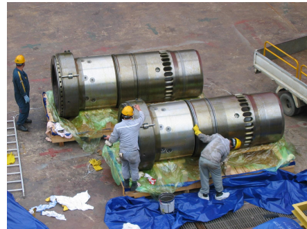
Cylinder liners at cleaning stage at shipyard.
