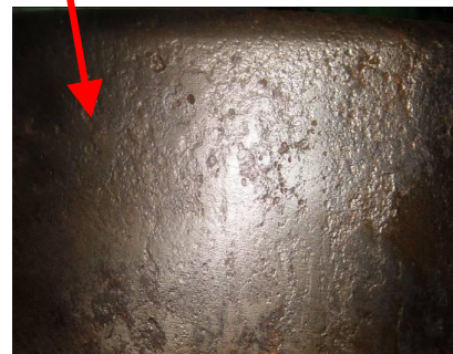
Repaired (cleaned of upper rust layer) cylinder liner (above) and piston crown (below) surface revealed that the pitting had been so heavy that the parts had to be replaced.
